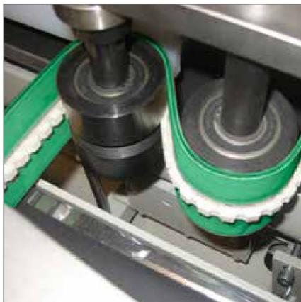
CHIORINO manufactures **profiles, guides and sidewalls** from special PVC and polyurethane compounds in various Sh.A hardnesses giving high flexibility and resistance to abrasion and oils.
